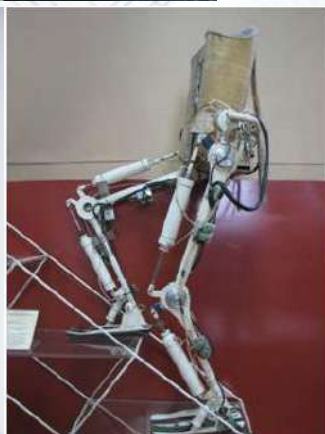
Most successful version of an active exoskeleton for rehabilitation of paraplegics developed in 1972 in Robotics Laboratory of Mihailo Pupin Institute
