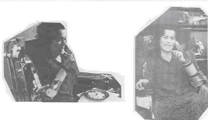
Successfully developed active arm orthosis for the rehabilitation of advanced cases of dystrophy and similar diseases. Controlled by means of a joystick. Made at the Mihailo Pupin Institute in 1982.
